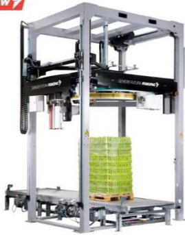
Genesis Futura HS 50 RPM machine 110 pallet loads per hour
